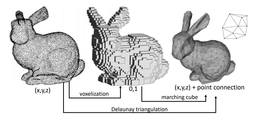
From left: The Stanford bunny model represented as *point cloud*, *voxel occupancy grid* and **mesh** [1]
